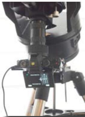
Then it's just a matter of diverting the Sun's image from the eyepiece to the camera through the dedicated photo port, which was done by flipping the lever shown in Figure 8.
