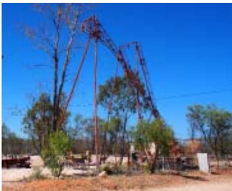
Lightning Ridge is well-known for its Black Opals which are mined underground. Outside the "Walk in Mine", a mine open to tourists, is the "Big Hoist". Built between 1985-1988 it was one of the biggest hoists in Lightning Ridge at that time. It was able to carry a large quantity of dirt, which reduced the amount of labour and effort required in moving dirt to the surface and trucking it out.
