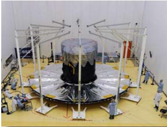
*Test Deployment of the 10 m Deployable Sunshield Array*
