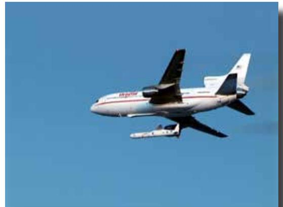
*NuSTAR was launched into a low-Earth, near-equatorial orbit on a Pegasus XL rocket from Kwajalein Atoll in the Marshall Islands. The Pegasus launch vehicle, built by Orbital Space Corporation, relies on a unique air-launch system with the rocket released at approximately 40,000 feet from the "Stargazer" L-1011 aircraft.*
