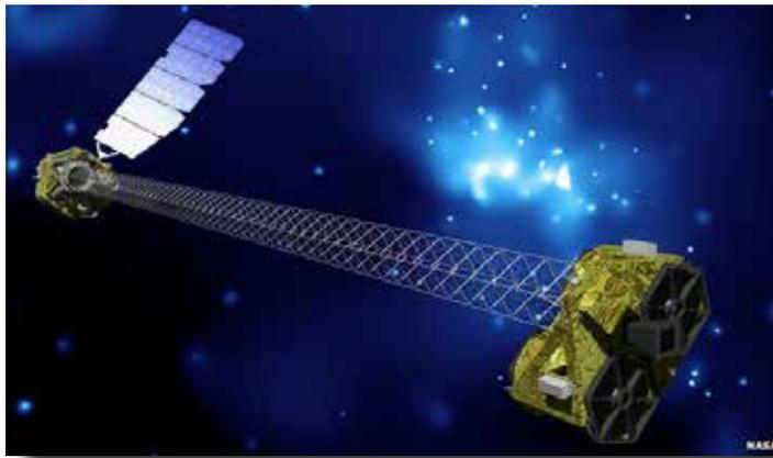
*Artist's concept of NuSTAR on orbit. NuSTAR's 10-metre mast separates the optics modules (right) from the detectors in the focal plane (left). NuSTAR has two identical optics modules in order to increase sensitivity.*
