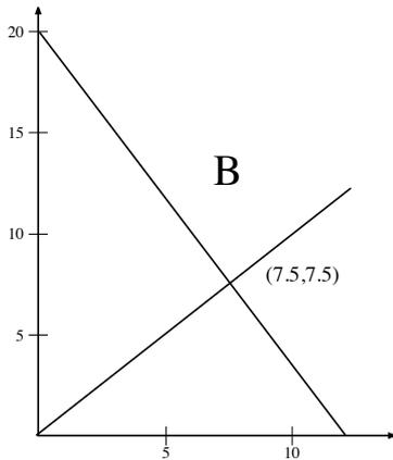
two capacities of 12 and 20 microfarads in series to make the equivalent of a single condenser with capacity 7.5 microfarads
