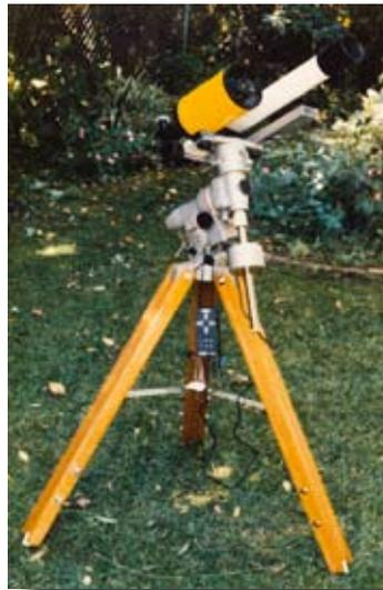
My 4 inch Schmidt-Cassegrain scope (yellow tube) with a cheap 60 mm refractor mounted alongside for guiding.
