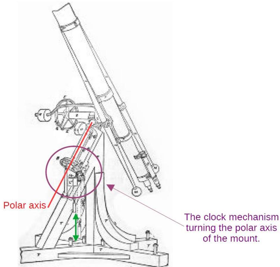
The design enabled the Telescope to be rotated around the polar axis with very little effort. The clock weights that were set before the observing run, the drive rotation rate controlled by a centrifugal regulator, was adjusted and set to keep the objects being viewed in the sky, centred in the eyepiece.
