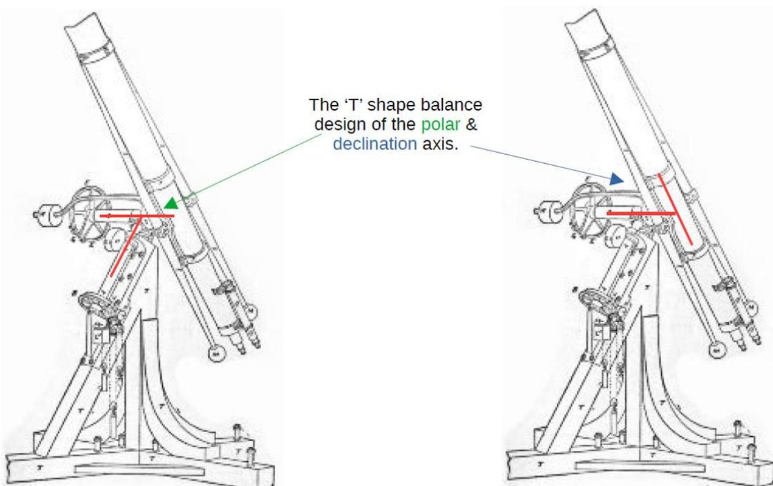
The mount's design of the balance of the Telescope on one side of the 'T' and a weight on the other side, enabled it to be driven by a clock mechanism. The mount's drive was the first in the world to automatically track objects in the sky.
