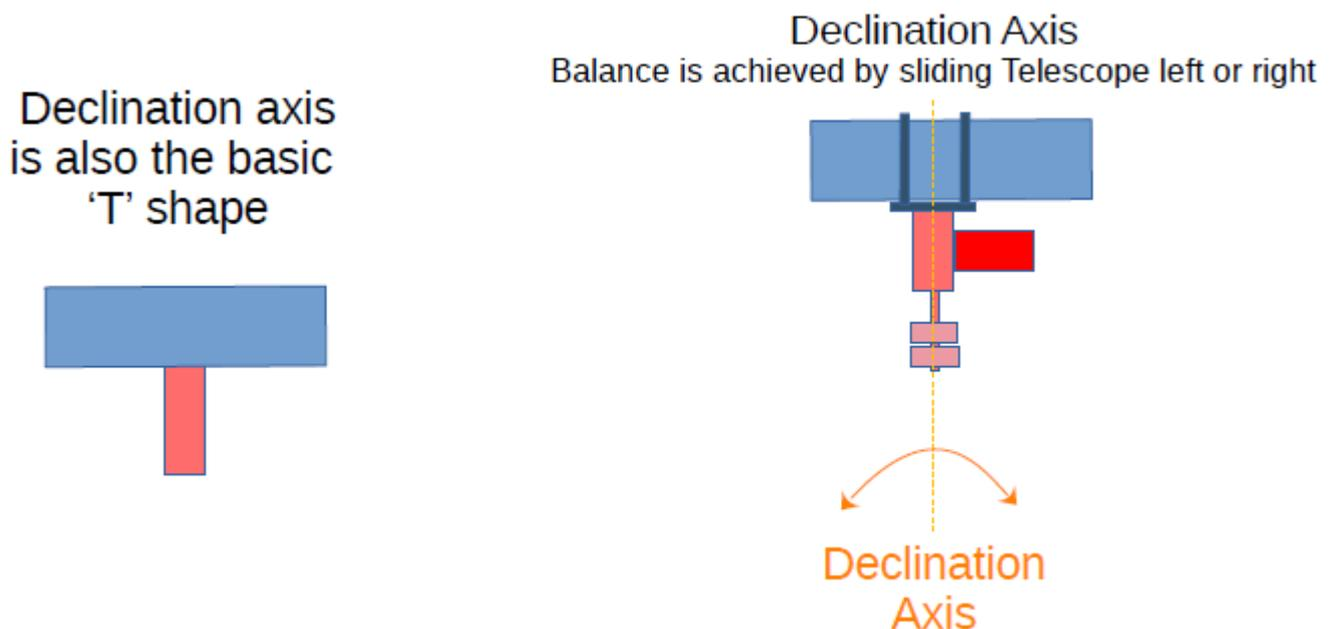
Balancing the declination axis is achieved not by moving weights as done in the polar axis, but by moving the Telescope mounting point to the mount until it's balanced.
