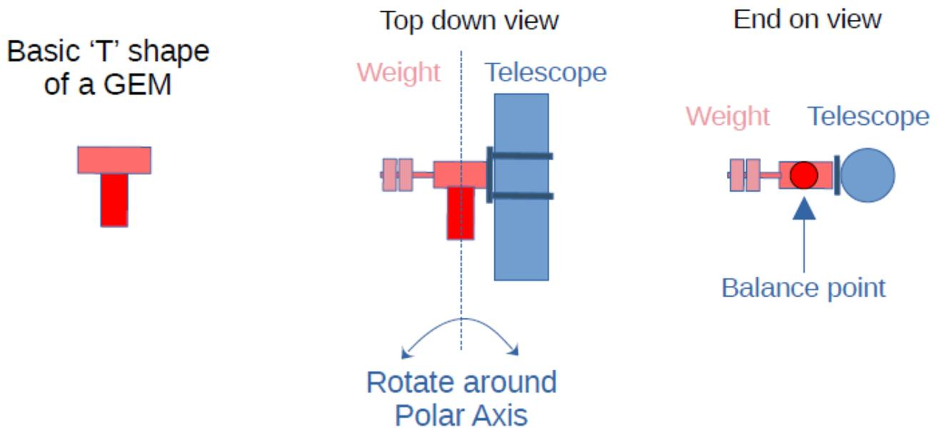
Rotating the Telescope around the Polar (or Equatorial) axis that is aligned with the celestial pole is the basic requirement of the Equatorial Mount. The position along the Equatorial axis is called the Right Ascension (or RA)
